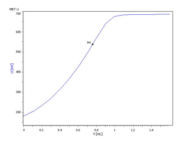
This Application Note describes the digestion of a cement sample and the photometric determination of iron according to DIN EN 196-2 by using the Optrode at 610 nm. Sulfosalicylic acid was used as indicator and EDTA as titrant.
