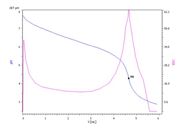
The automated system **Basic water analysis** determines conductivity, pH value, and alkalinity in all kind of water samples. The high degree of automation (e.g., automated sample addition, automated calibration as well as automated titer and cell constant determination) minimizes errors and guarantees an outstanding reproducibility.
