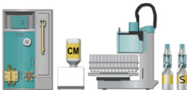
Figure 1. Setup for drinking water testing using a 930 Compact IC Flex with automatic KOH eluent generation (948 Continuous IC Module, CEP), an 858 Professional Sample Processor, and the Metrohm intelligent Partial-Loop Injection Technique (MiPT).
