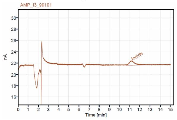
Anion chromatogram of 1  $\mu$ g/L iodide, acquired by OpenLab CDS.
