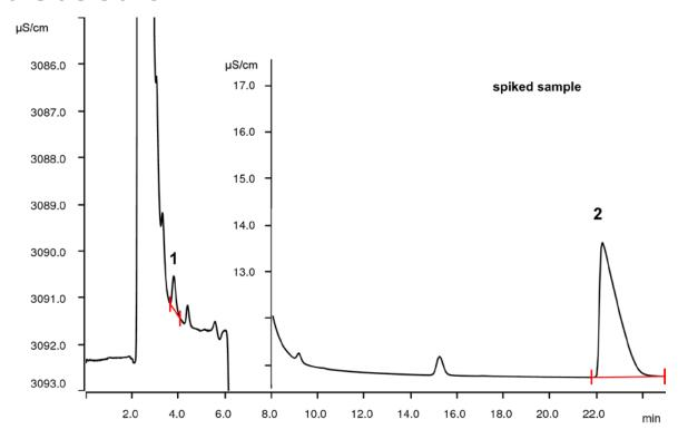
Determination of arsenic in dust from a waste incineration plant is performed. This is required as the environmental risk depends on the degree of oxidation of the arsenic species. Due to the different  $pK_a$  of the respective anions, arsenite requires non-suppressed conductivity detection, while arsenate is determined best with suppression. The determination of both species is achieved by switching the suppressor in and out respectively.
