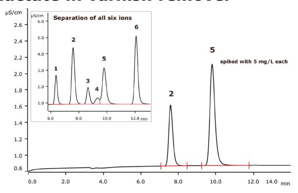
Glycolate and lactate have to be determined in a dual phase varnish remover. Analyzed is only the upper aqueous phase. The separation is achieved on a Metrosep A Supp 16 - 250/4.0 column. The eluent composition is adapted to get a sufficient separation of glycolate and lactate without interference by formate and acetate. Conductivity detection after sequential suppression is applied.
