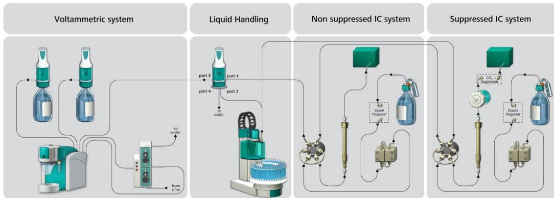
The liquid-handling Dosino fills the loops of both ion chromatographs and transfers the sample to the VA measuring vessel.
