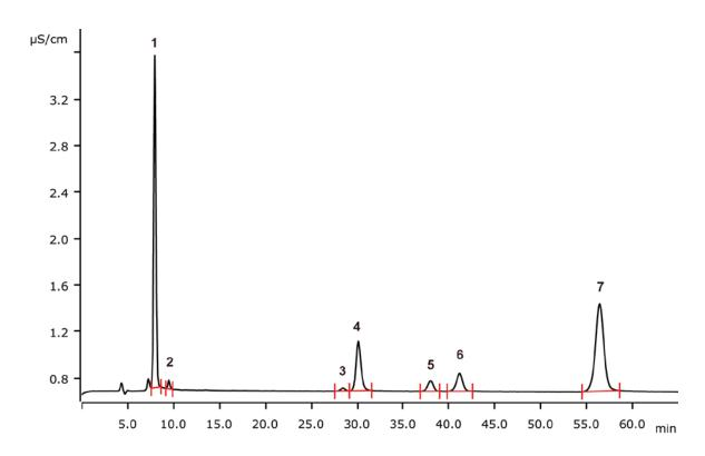
Natural gas production requires the removal of acidic gases (e.g.,  $H_2S$  and  $CO_2$ ). These are removed by treatment with alkanolamines or alkylalkanolamines such as methyldiethanolamine (MDEA). In these solutions, heat stable salts (HSS) may accumulate and need to be monitored. The analysis of the heat stable salts in MDEA solutions is performed on a Metrosep A Supp 5 - 250/4.0 column with conductivity detection after sequential suppression.
