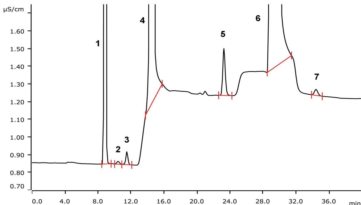
Trace organic acids besides high concentrations of standard anions are difficult to analyze because the peaks of the acids disappear under those of the standard ions. A simple Dose-in Gradient ensures baseline separation of acetate, formate, and fluoride. Similarly, oxalate elutes well after sulfate. Separation is performed on a Metrosep A Supp 7 - 250/4.0 column with subsequent conductivity detection after sequential suppression.
