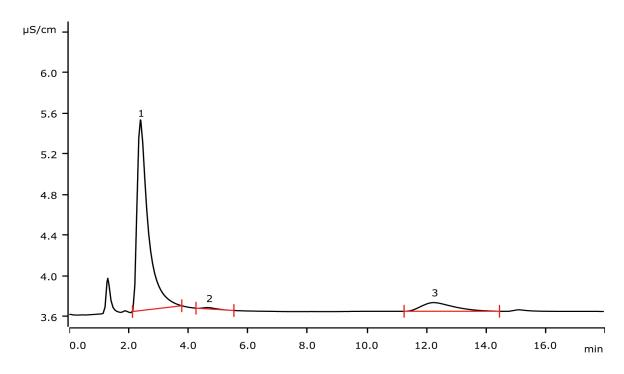
Aromatic dicarboxylic acids such as terephthalic (TPA), isophthalic (IPA), and 5-sulfoisophthalic acid (SIPA) are important monomers for producing polyesters and alkyd resins. The monomer ratio is crucial for the polymerization process. The separation of the late-eluting components is achieved within 15 min on a short Metrosep A Supp 15 - 50/4.0 column applying a high eluent concentration and a high flow rate.
