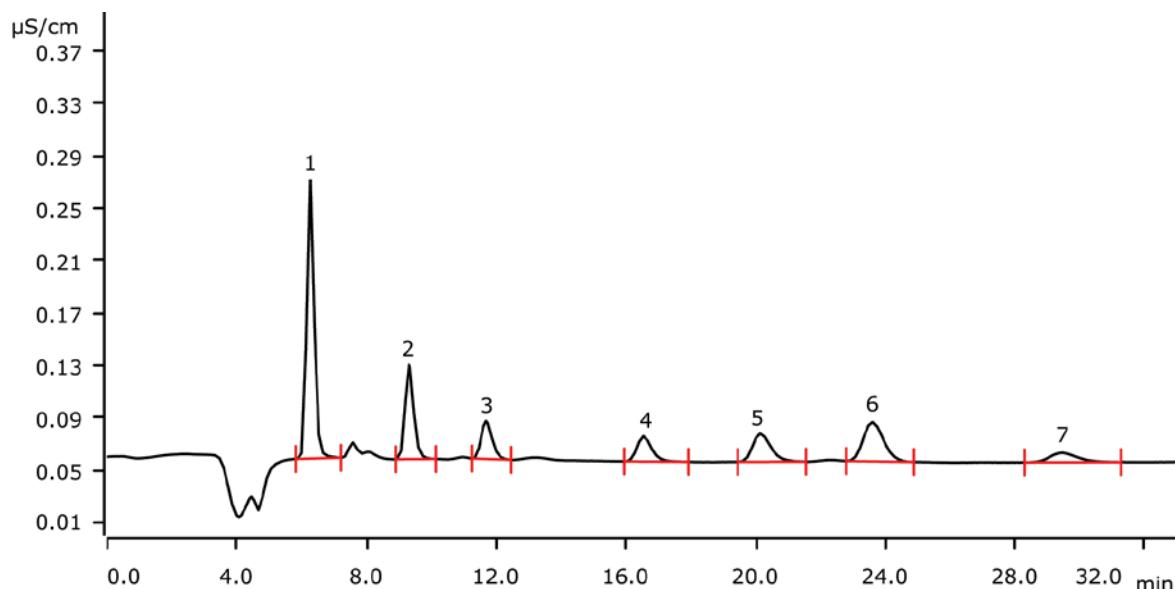
Intelligent Preconcentration Technique with Matrix Elimination (MiPCT-ME) is used for trace determination of the seven standard anions. On a microbore Metrosep A Supp 16 - 250/2.0 column, the analysis is concluded within 33 minutes with high recovery rates. The detection limits are in the low ng/L range (calculated by MagIC Net) using a preconcentration volume of 2000 µL.
