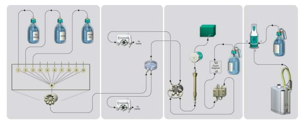
The samples were injected through port 1, the check standard was injected through port 3, standards for calibration were injected through port 4 and ultrapure water was supplied through port 2 of the 10-port selector valve of the 942 Extension Module Vario LQH.
