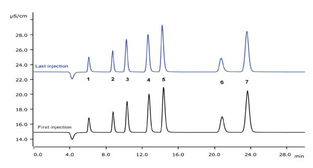
The stability of the microbore version of the Metrosep A Supp 5 - 250/2.0 has been tested under lab conditions. For six consecutive days, two series of injections were done –  $9 \times$  tap water,  $3 \times$  check standard,  $6 \times$  tap water –; on the  $7_{th}$  day, the system was shut down. The instrument was running for over 12 weeks with a total of 2650 injections. The excellent data reproducibility underlines the very stable column performance.
