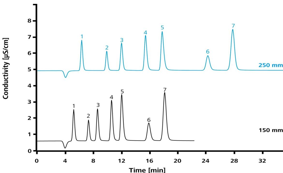
The microbore version of the Metrosep A Supp 5 is available in 150 and 250 mm length. The standard ions are separated within 20 and 29 minutes, respectively. Besides the good separation and short run time, the microbore column impresses with the very low eluent consumption.
