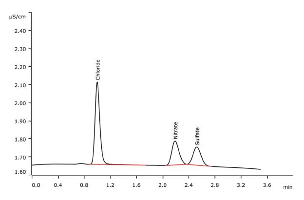
Fast IC means high sample throughput on short columns with relatively high flow rates and strong eluents. Applied to drinking water analysis, this means: determination of chloride, nitrate, and sulfate within three minutes on a Metrosep A Supp 10 - 50/2.0.
