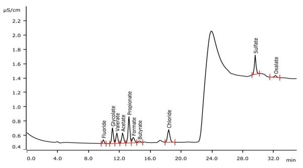
The separation of short-chain organic acids from fluoride and chloride requires diluted eluents. These weak eluents, however, induce long retention times for divalent anions. Adding a stronger eluent later in the run by use of a Dose-in Gradient makes these anions elute sooner. An advantage of the Dose-in Gradient is that it does not require multiple high-pressure pumps or proportioning valves.
