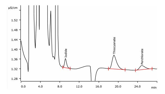
Anion analysis in milk requires a sophisticated sample preparation to avoid column fouling by fats or proteins. Here Metrohm Inline Dialysis is the perfect automated technique. In dairy products, iodide, thiocyanate, and perchlorate need to be determined regularly for health and hygiene reasons. This application allows for the first time to analyze these three components in this matrix within one run.
