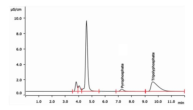
Whitening toothpaste often contains polyphosphates to remove stains. The analysis of these polyphosphates requires a high-pH hydroxide eluent. The high eluent concentration is suppressed by the high-capacity suppressor MSM-HC.
