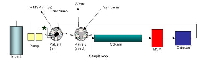
Step 1: Injection of the sample on «Valve 2»
