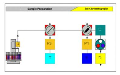
The retained anions are transferred in counterflow with the eluent to the analytical column.
