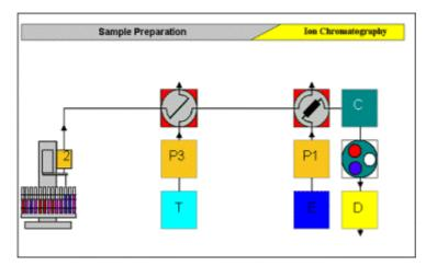
The sample in the loop is transferred to the preconcentration column using transfer solution and the matrix is eliminated.
