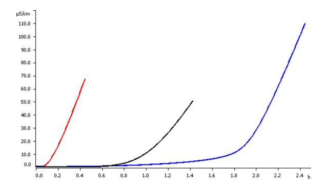
Determination of the thermostability of polyvinyl chloride (PVC) using the dehydrochlorination procedure at 180 °C. Comparison of the thermostability of pure PVC polymer, blended PVC (blended with stabilizer, plasticizer, filler) and blended PVC after processing.
