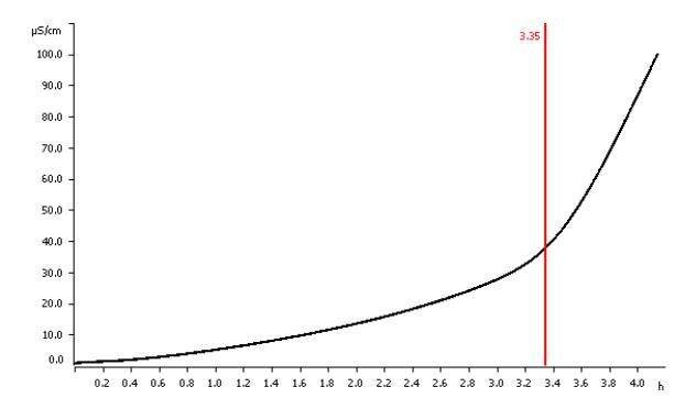
Determination of the oxidation stability of rapeseed oil using the Rancimat method.
