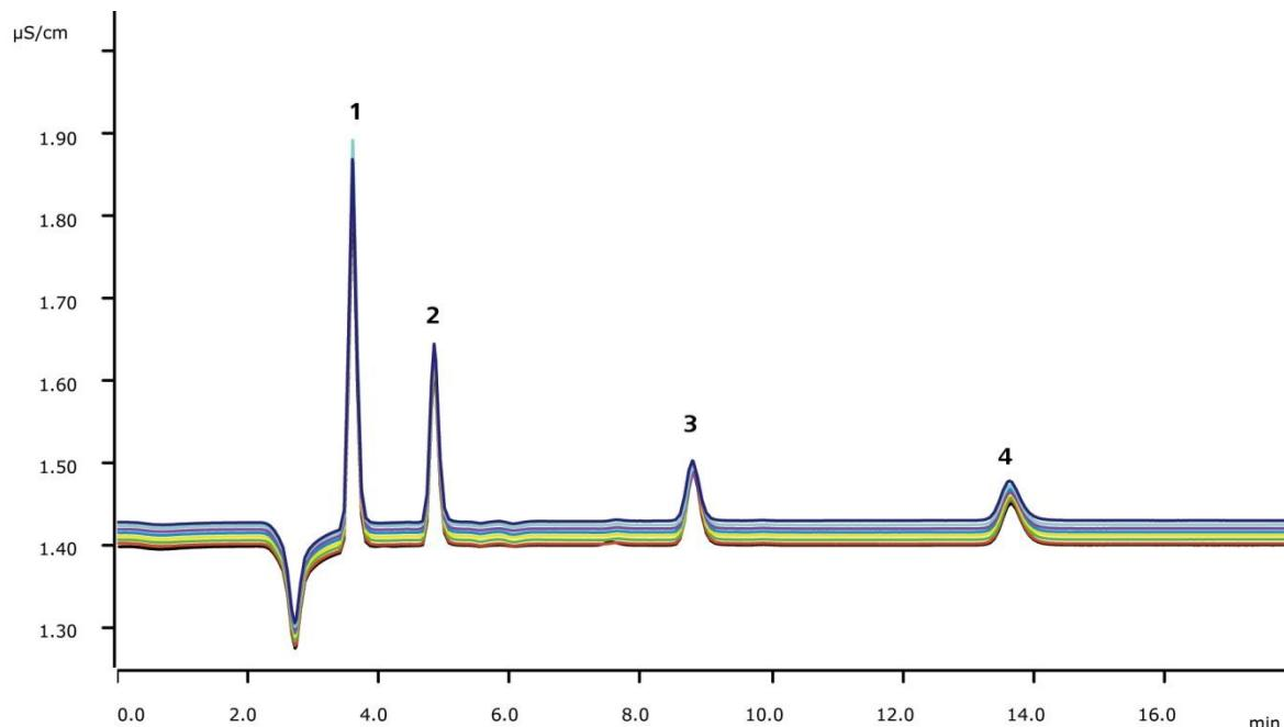
A setup that allows online sampling is crucial for immediate and contamination-free analysis of power plant water samples. This application recommends a setup that facilitates simultaneous anion/cation determinations. Automated inline sample preparation combines variable preconcentration (MiPCT) and calibration with a single multi-ion standard. AN-Q-004 displays the respective cation results.
