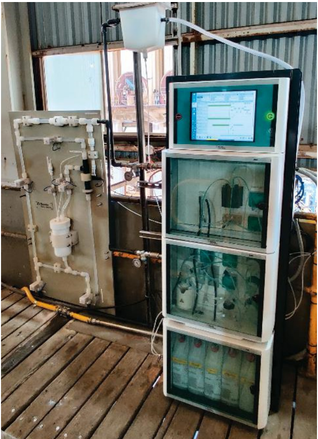
Figure 2. 2060 TI Process Analyzer with preconditioning panel in a zinc refining plant.
