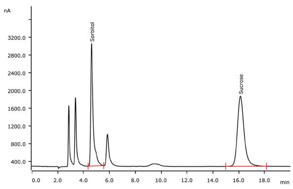
Polyols and sugar components in soaps increase the stability and size of bubbles and foam. A typical soap ingredient is glycerol. But sugar alcohols and sugars are used as well. The determination of sorbitol and sucrose in a transparent soap is achieved on a Metrosep Carb 2 - 150/4.0 column with subsequent pulsed amperometric detection (PAD).
