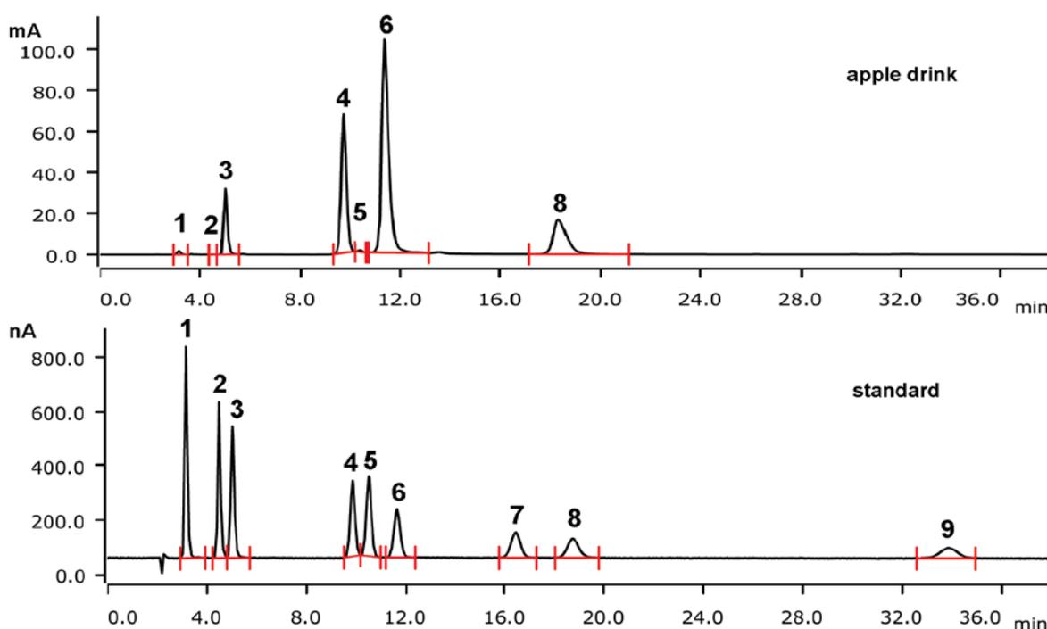
Sugars and sugar alcohols in food are separated on a Metrosep Carb 2 - 150/4.0 column and detected with pulsed amperometric detection. The method is applied to an apple drink.
