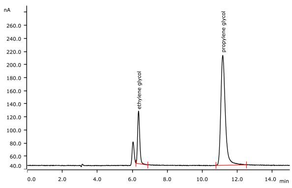
Glycol solutions are used in antifreeze, e.g., in automobiles. Because of its toxicity, monoethylene glycol (MEG) is being increasingly replaced by propylene glycol. This Application Note shows the separation and quantification of both glycols. Separation is achieved on a Metrosep Carb 2 - 250/4.0 column. As glycols show no conductivity and have no chromophore, pulsed amperometric detection (PAD) is the detection mode of choice.
