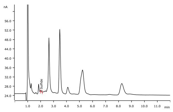
Sulfide determination in wastewater by ion chromatography is performed using an alkaline eluent and amperometric detection. The sample needs to be set to an alkaline pH as well to ensure that the sulfide is stable. DC amperometric detection at a silver electrode offers high selectivity and sensitivity. Separation takes place on a Metrosep A Supp 10 - 100/4.0 column.
