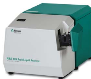
Fig. 1: The NIRS XDS RapidLiquid Analyzer was used for spectral data acquisition over the full range from 400 nm to 2500 nm.
