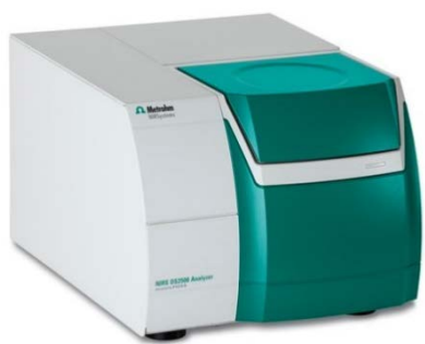
Fig. 1: The NIRS DS2500 Analyzer was used for spectral data acquisition over the full range from 400 nm to 2500 nm.
