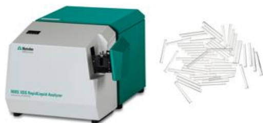
Fig. 1: A NIRS XDS RapidLiquid Analyzer equipped with 4 mm NIRS disposable glass vials were used to generate the spectral data in true transmission mode over the full wavelength range (400–2500 nm).
