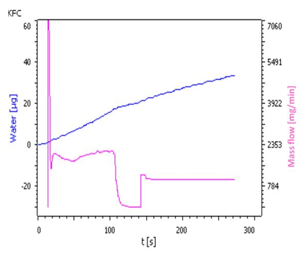
This Application Note describes the automated determination of the water content in liquid chloromethane (methyl chloride) using the 875 KF Gas Analyzer.
