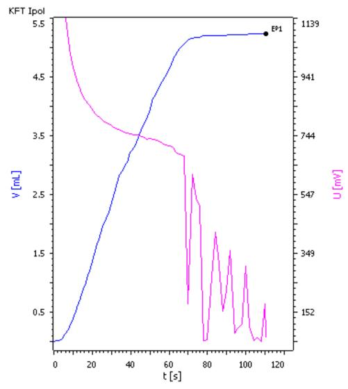
This Application Note describes the automated determination of the water content in tooth paste using volumetric Karl Fischer titration (MATi 10).
