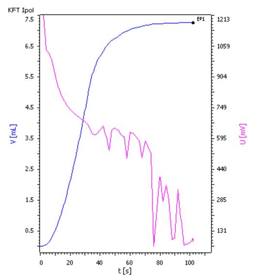
This Application Note describes the automated determination of the water content in sodium acetate using volumetric Karl Fischer titration (MATi 10).
