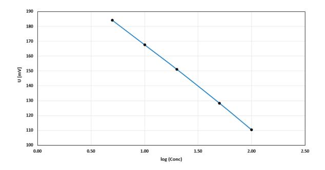
In the synthesis of certain dyes, sodium chloride is a byproduct. The content of chloride is therefore an important parameter. This application note describes the determination of the chloride content in dye by standard addition using a Cl<sup>-</sup> ion-selective electrode.
