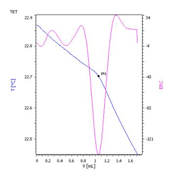
The reliable knowledge of the accurate acid number for crude oil is important for the determination of the price of crude oil. Additionally, by monitoring the acidity of crude oil and the associated process oils unexpected shutdowns can be prevented and thus expensive treatment chemicals preserved. The determination of the acid number in crude oil and various gas oil samples by catalytic thermometric titration is described here.
