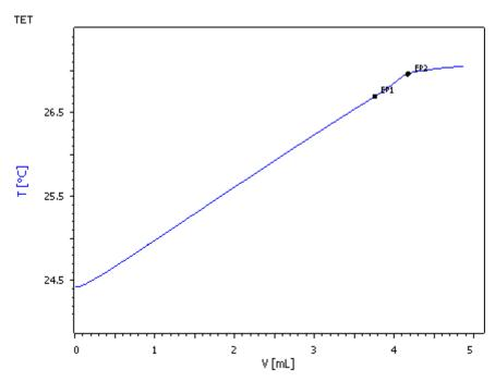
A mix of hydrochloric and hydrofluoric acid can be determined in ethanol- and acetonitrile-containing etching baths by thermometric titration. In the titration curve, two different endpoints can be detected: they are used to quantify the respective acid.
