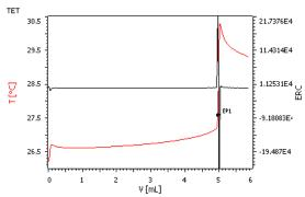
CETT titration of piperidine with 0.1 mol/L CF<sub>3</sub>SO<sub>3</sub>H
