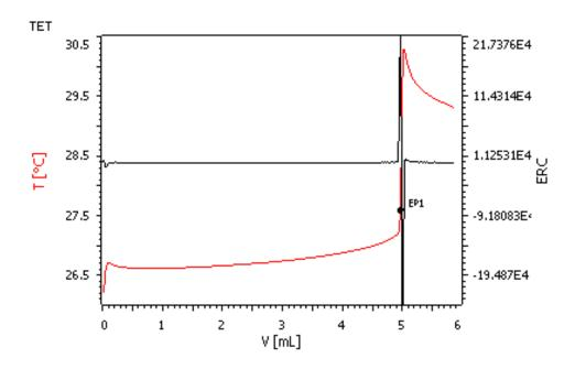
Weak organic bases soluble in nonaqueous solvents (including nonpolar solvents) may be determined by titration with strong acids such as anhydrous perchloric or trifluoromethanesulfonic acid in glacial acetic acid. The endpoint of such titrations may be determined thermometrically, if a suitable thermometric endpoint indicator is used. Isobutyl vinyl ether (IBVE) has been found to be very suitable for this purpose.
