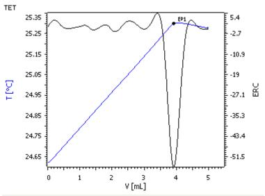
Fig. 2. Titration of sulfuric acid component with  $c(BaCl_2) = 1 \text{ mol/L}$
