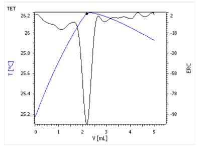
Fig. 1. Thermometric titration of total fluoride concentration with  $c(AI(NO_3)_3) = 0.5 \text{ mol/L}$
