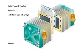
Figure 3 – Schematic overview of a fuel cell stack.
