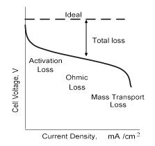
Figure 2 - i-V curve of a fuel cell showing the individual losses
