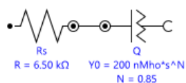
Figure 1 – Equivalent circuit describing the interface between a good ion conductor and an inert electrode.
