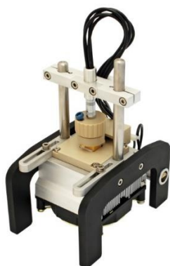
Figure 3 – Overview of the cell holder and the electrochemical cell.
