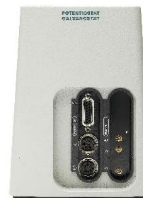
Figure 1 – The Autolab PGSTAT204, equipped with the FRA32M.
