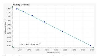
Figure 2 - Linear sweep voltammetry profiles (top) from the disk electrode at various rotation rates; the potential value for the Levich and Koutecký-Levich analyses are indicated. Levich (middle) and Koutecký-Levich (bottom) plots.
