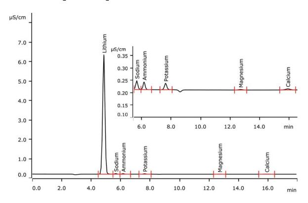
Lithium hexafluorophosphate (LiPF<sub>6</sub>) is used as electrolyte in rechargeable batteries. Particularly the high solubility in non-polar solvents and the non-coordinating character of the hexafluorophosphate anion make it ideally suited for lithium-ion cells. This application describes the determination of trace cations in the salt applying conductivity detection after sequential cation suppression.
