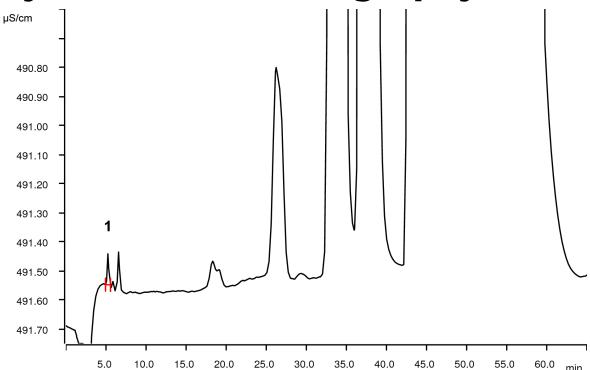
Bicine (2-(Bis(2-hydroxyethyl)amino)acetic acid) is a corrosive component. It has to be avoided in acidic gas sweetening solvents. These solvents are based on organic amines. Bicine is amphoteric, holding a carboxylic and an amine group. Under the applied conditions, the amine groups are at least partially protonated and therefore may be separated by cation chromatography. The detection mode is direct conductivity detection.
