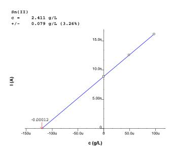
Determination of tin(II) by anodic stripping voltammetry
