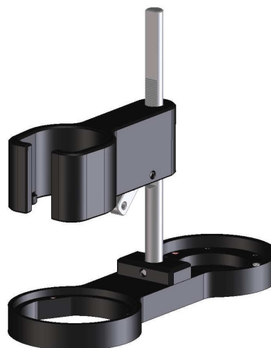
Figure 29: 6.9914.140 Robotic arm with holder for titration head and Polytron, right swinging. Aggregate in the center of the titration beaker (used in combination with a 786 Swing head).
