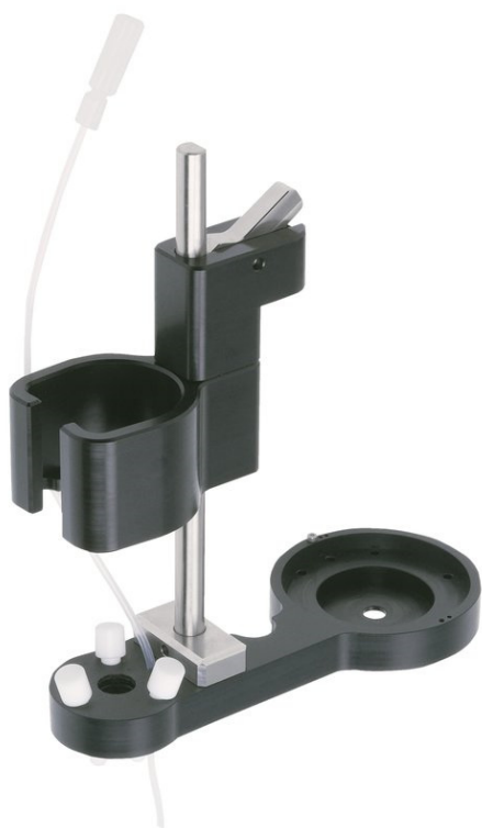
Figure 28: 6.1462.250 Robotic titration arm with Polytron holder, left swinging (used in combination with 786 Swing Head) and equipped with one buret tip for solvent addition and three spray nozzles for cleaning.
