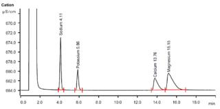
For the calibration, the average peak areas of 3 injections were evaluated. Within the concentration range of 0.25–20 mg/L, a quadratic curve type was used for evaluation.
