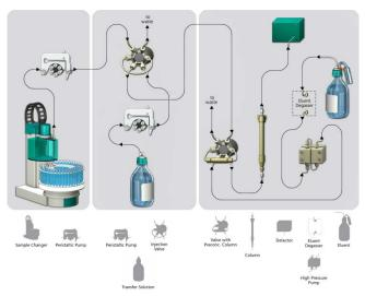
Prepare and degas an eluent suitable for the column you want to use (see column leaflet). For Metrosep C 4 - 150/4.0 a solution of 1.7 mmol/L HNO<sub>3</sub> / 0.7 mmol/L dipicolinic acid (DPA, 2,6-Pyridinedicarboxylic acid) is adequate.
