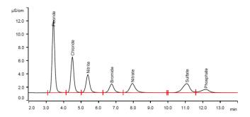
For the calibration, the average peak areas of 3 injections were evaluated. Within the concentration range of 1 - 20 mg/L, a quadratic curve type was used for evaluation. Correlation coefficients and standard deviations are listed in the following table. The calibration curve for fluoride is shown as an example.
