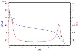
Fig. 2: Titration curve of the hydroxyl number determination according to ASTM E1899 for a polypropylene glycol
