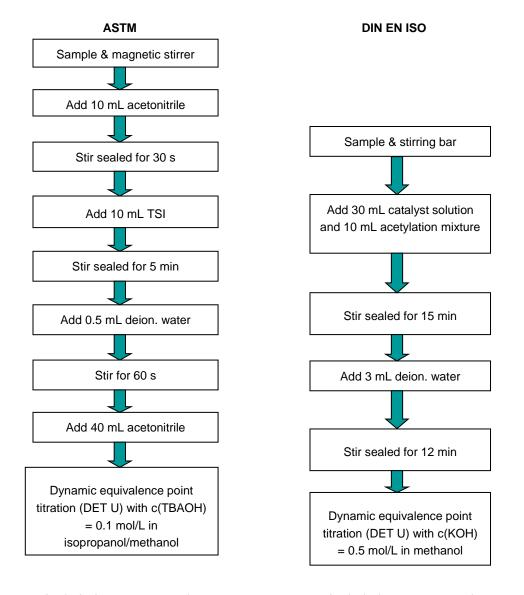
Analysis time approx. 12 minAnalysis time approx. 40 minFig 1:Comparison of the two analysis methods including the approximated titration time for each method.
