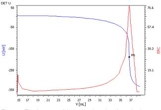
Fig. 3: Titration curve of the hydroxyl number determination according to DIN EN ISO 4629-2 for an oxooil
