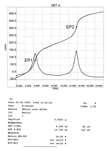
*Fig. 2:* Titration curve with first derivative and result report of a typical betain titration with perchloric acid (716 DMS Titrino with Metrodata TiNet 2.0).
