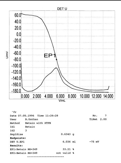
*Fig. 1:* Titration curve with first derivative and result report of a typical betain titration with sodium tetraphenylborate (716 DMS Titrino with Metrodata TiNet 2.0).
